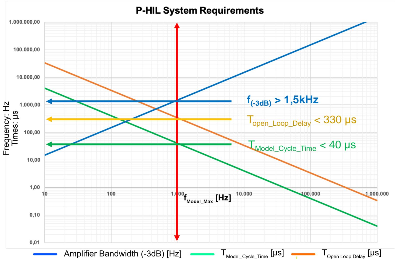
Example:  $f_{\text{Model\_max}} = 10 \text{ kHz}$
