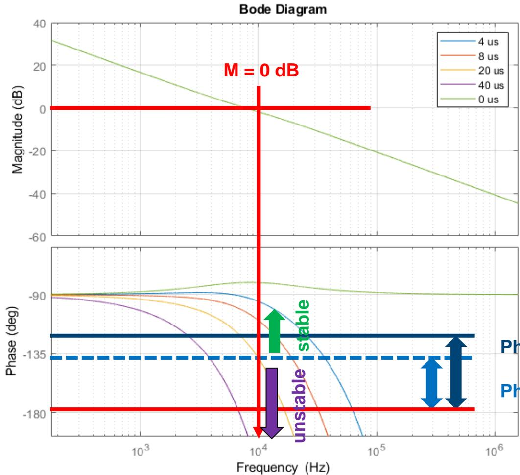
Phase Reserve Optimal:  $\phi \geq 60^\circ$
